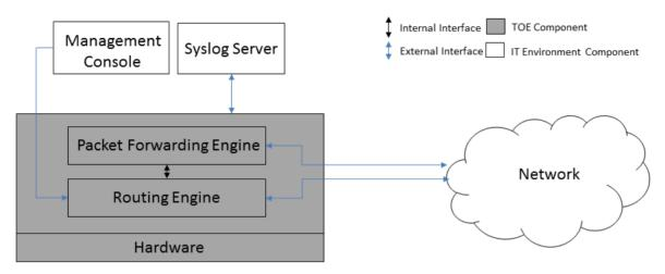
The physical boundary for the SRX1500 is shown in the figure below.
